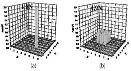
Fig. 10. Experimental results of the tactile sensor; (a)point load detection, and (b)distributed load detection.
