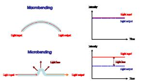
Fig.1. Microbending effect of the optical fiber.
