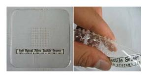
Fig. 9. Fabricated prototype tactile sensors and its flexibility
