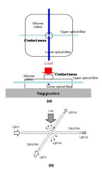
Fig. 2. (a) Structure of the taxel, (b) the microbending effect of the optical fibers in the silicon rubber.
