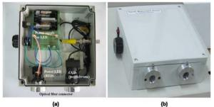
Fig. 5. Optical measuring system of this tactile sensor system; (a) The interior, (b) The exterior
