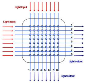
Fig. 7. Schematics of the tactile sensor using microbending fiber optic sensors with the fabric structure
